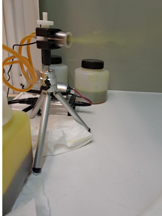
Figure 10: View of the generator and a solution containing fluorescein and glycerol during a test in the laboratory in a fume hood
