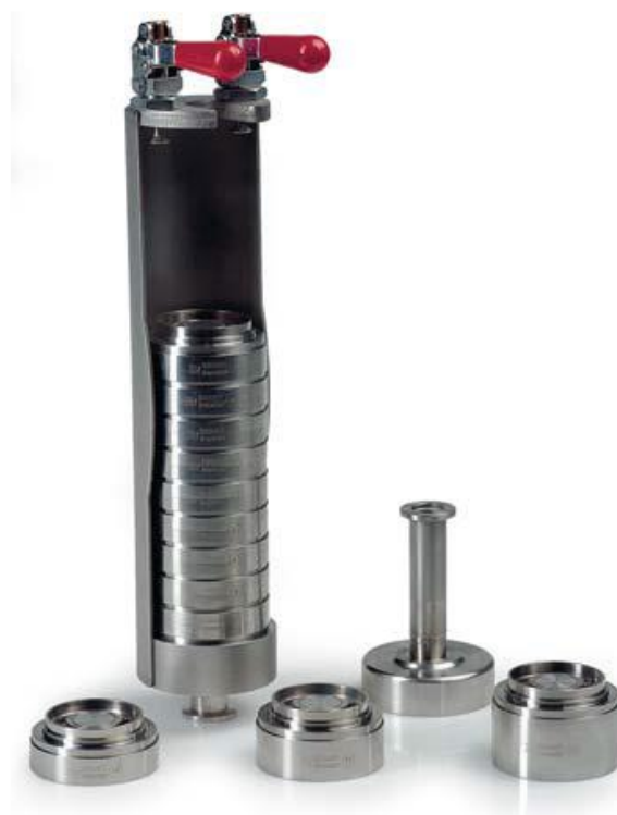
Figure 7: View of an LPI DEKATI Inc. (source: DEKATI.com)
