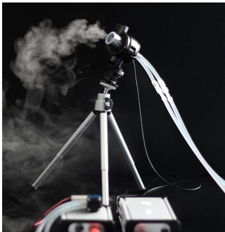
Figure 5: View of the TEKCELEO MICRONICE® 12 µm generator (P&S-360) in operation (source: TEKCELEO.com)
