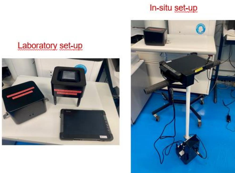
Figure 7 Modified MAUD system for measurement of large surfaces.
